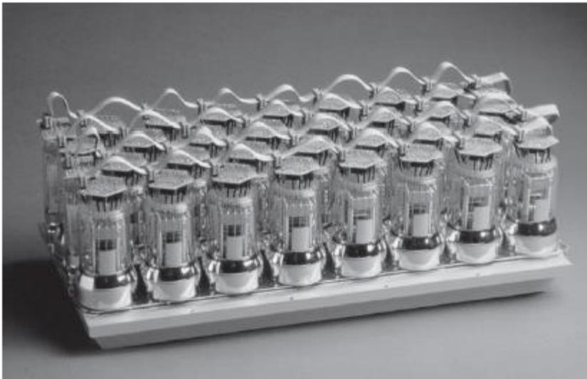
**E 13-3** A rectangular gamma camera detector with the cover removed showing the photomultiplier (PM) tubes mounted on the NaI(Tl) crystal. In this example, the gamma camera detector measures  $50 \times 15$  cm and is read out by tubes 5 cm in diameter. This is a digital camera in which each of the PM tube outputs is individually digitized. (by Dr. Joel Karp, University of Pennsylvania, Philadelphia, PA.)
