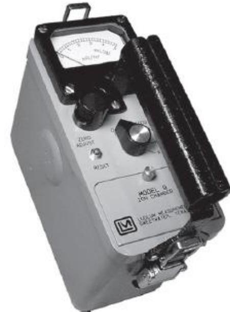
**FIGURE 7-3** A battery-powered radiation survey meter. An ionization chamber is contained in the base of the unit, with the entrance window on the bottom face of the device (not shown). The meter indicates radiation level. The rotary switch is used to select different scale factors. (Courtesy Ludlum Measurements, Inc., Sweetwater, TX.)
