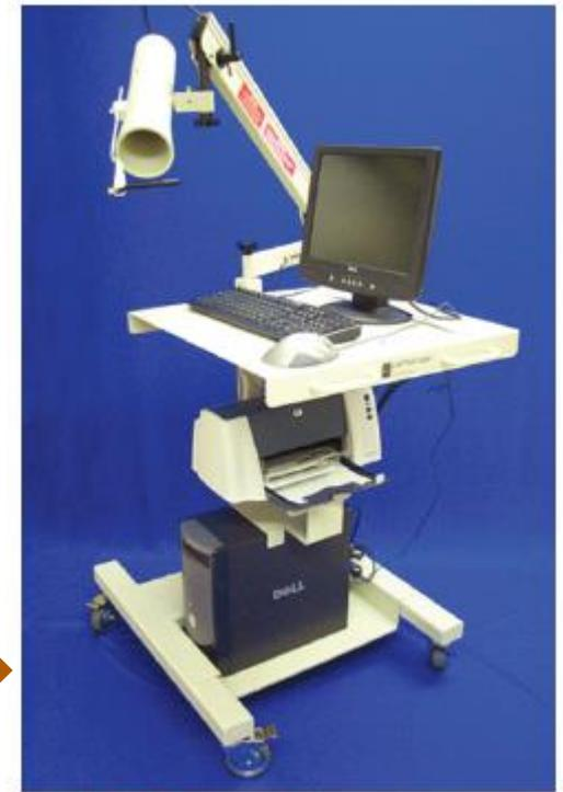
FIGURE 12-19 Typical NaI(Tl) probe system for measuring thyroid uptake of radioactive iodine. (Courtesy Capintec, Inc., Ramsey, NJ.)
