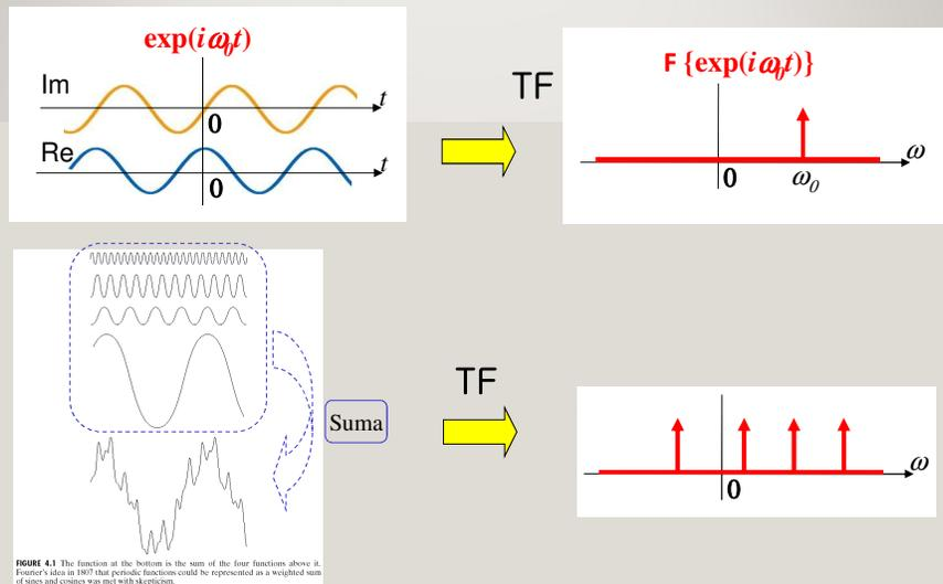
FIGURE 4.1 The function at the bottom is the sum of the four functions above it. Fourier's idea in 1807 that periodic functions could be represented as a weighted sum of sines and cosines was met with skepticism.
