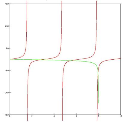
The green curve is  $\frac{-1}{\sqrt{z_0^2/z^2-1}}$  and the red curve is  $\tan z$ . In this case we can see there are 3 intersections, so here there are 3 bound states. The precise values of the energies can be found by solving the equation numerically
