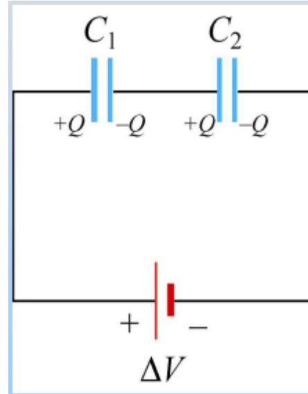
$$\Delta V_1 = \frac{Q}{C_1}, \quad \Delta V_2 = \frac{Q}{C_2}$$
