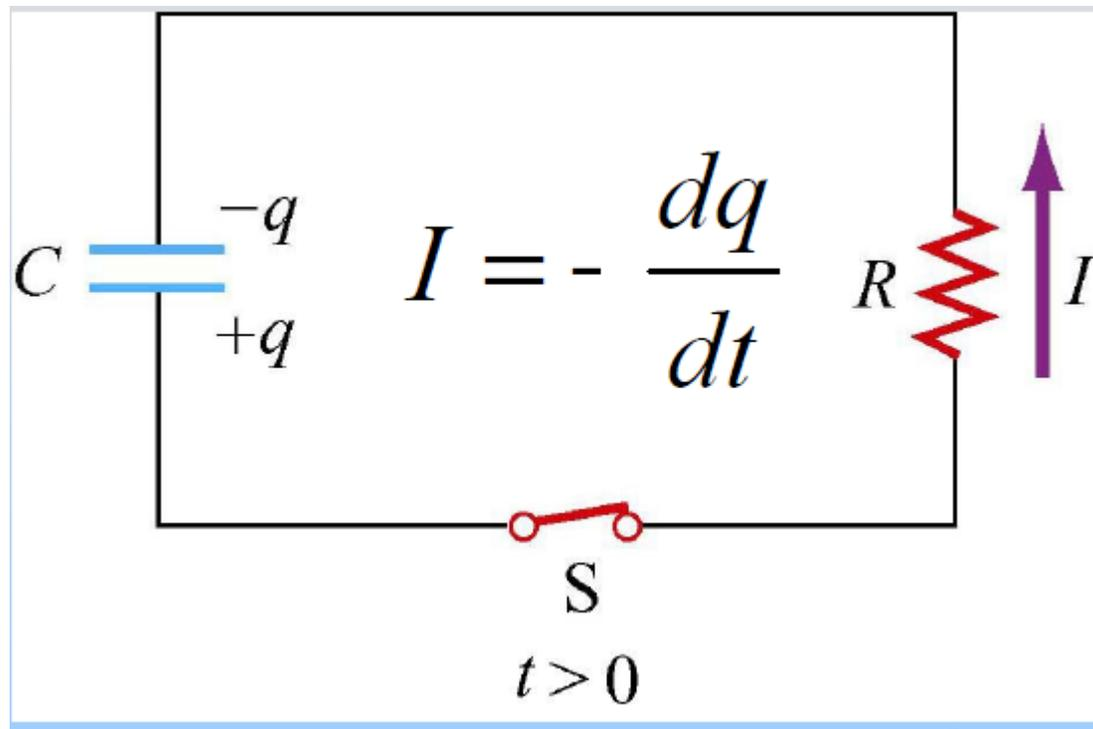
$$\sum_i \Delta V_i = \frac{q}{C} - IR = 0 \quad \sum_i \Delta V_i = \frac{q}{C} + \frac{dq}{dt} R = 0$$
