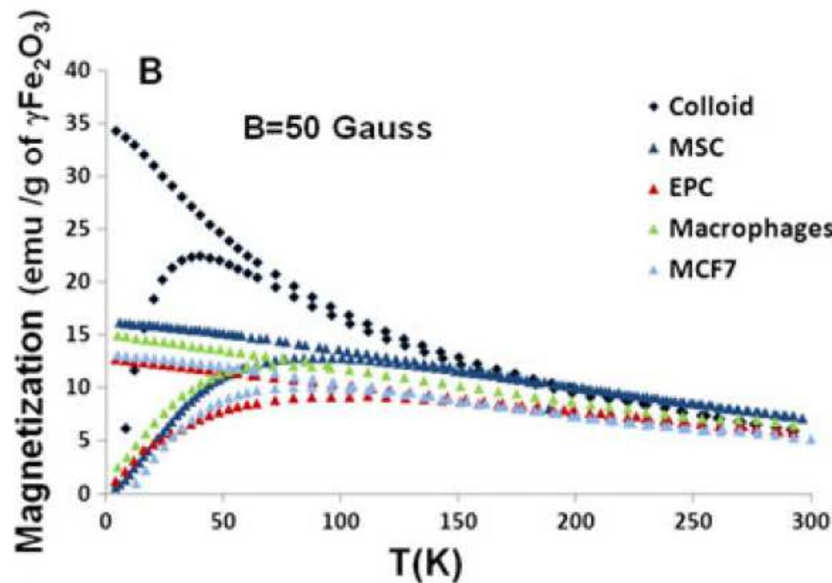
Magnetic and NMR characterization of nanoparticles (NPs) internalized in EPC (13.8 pg iron per cell), MSC (30.5 pg per cell), macrophages (13.1 pg per cell), MCF7 (3.2 pg per cell) or PC3 (2.7 pg per cell) in comparison with the corresponding colloid.
