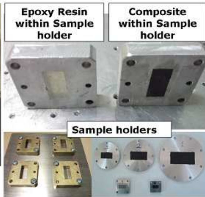
Measurements of Scattering parameters S_{nm} and Dielectric parameters computation \mu \epsilon
