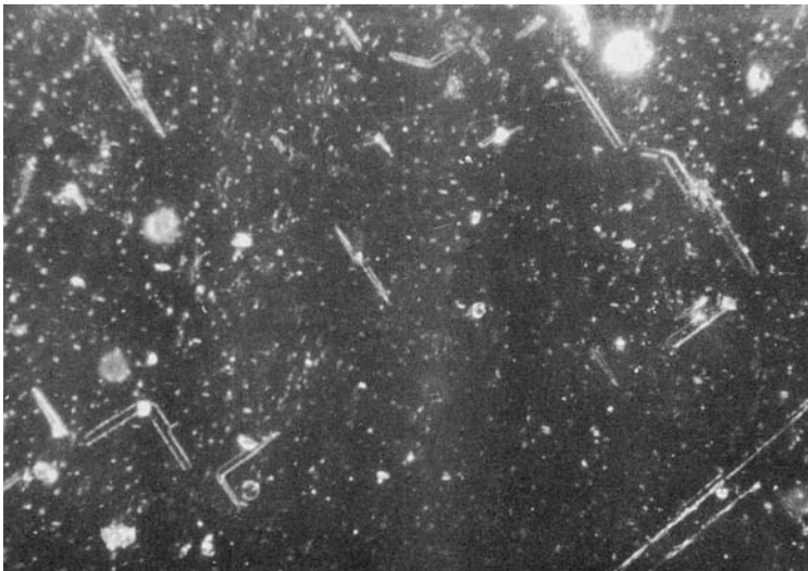
Fig. 9.28 Spike domains at inclusions in an Fe + 3% Si crystal.
