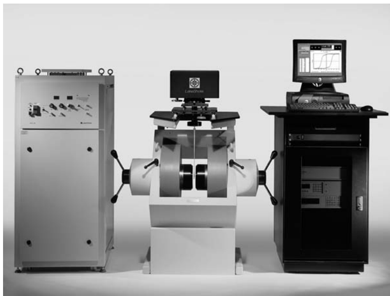
Fig. 2.10 Commercial electromagnet (center). Power supply at left, control and measurement equipment on right. Courtesy Lake Shore Cryotronics, Inc.
