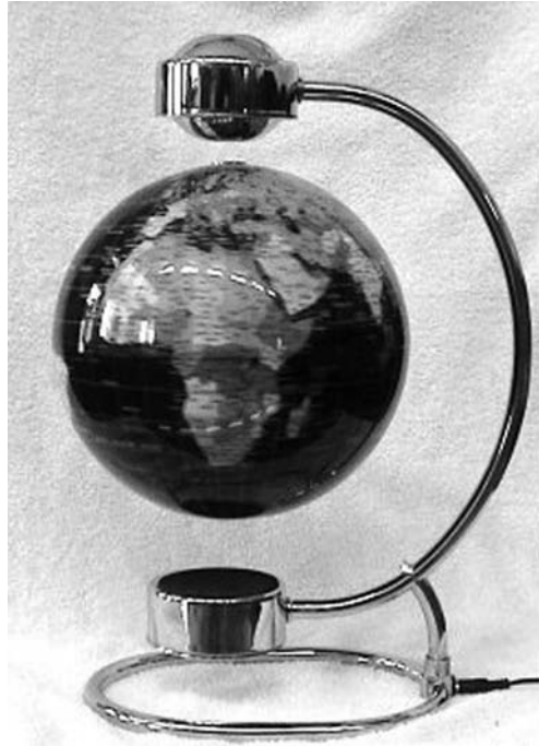
Fig. 14.21 Floating globe using magnetic suspension with feedback.
