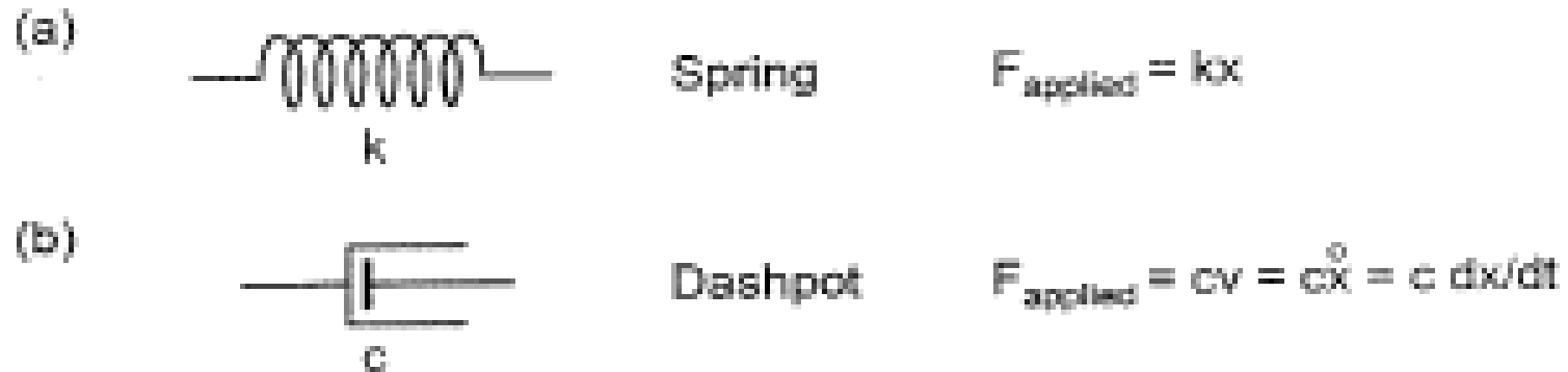
Fig. 4.43. (a) Ideal (or perfect) spring and (b) ideal (or perfect) dashpot. These are the two basic building blocks used in modeling the mechanical response of materials
