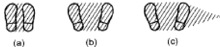
Fig. 3.6. A standing person is stable when her center of mass is over the cross-hatched region spanned by her feet, as shown here with her feet (a) together, (b) apart, (c) and apart, with stability also provided by a cane or crutch. (Based on [110])
