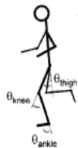
Fig. 3.1. One set of conventions for hip (thigh), knee (lower leg), and ankle (foot) angles. Other conventions are also used, such as with the thigh angle being relative to the vertical and the ankle angle defined as 90^\circ less than here. (Based on [150])
