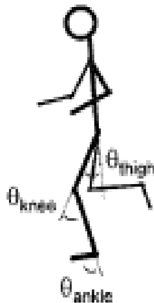
Fig. 3.1. One set of conventions for hip (thigh), knee (lower leg), and ankle (foot) angles. Other conventions are also used, such as with the thigh angle being relative to the vertical and the ankle angle defined as 90^\circ less than here. (Based on [150])
